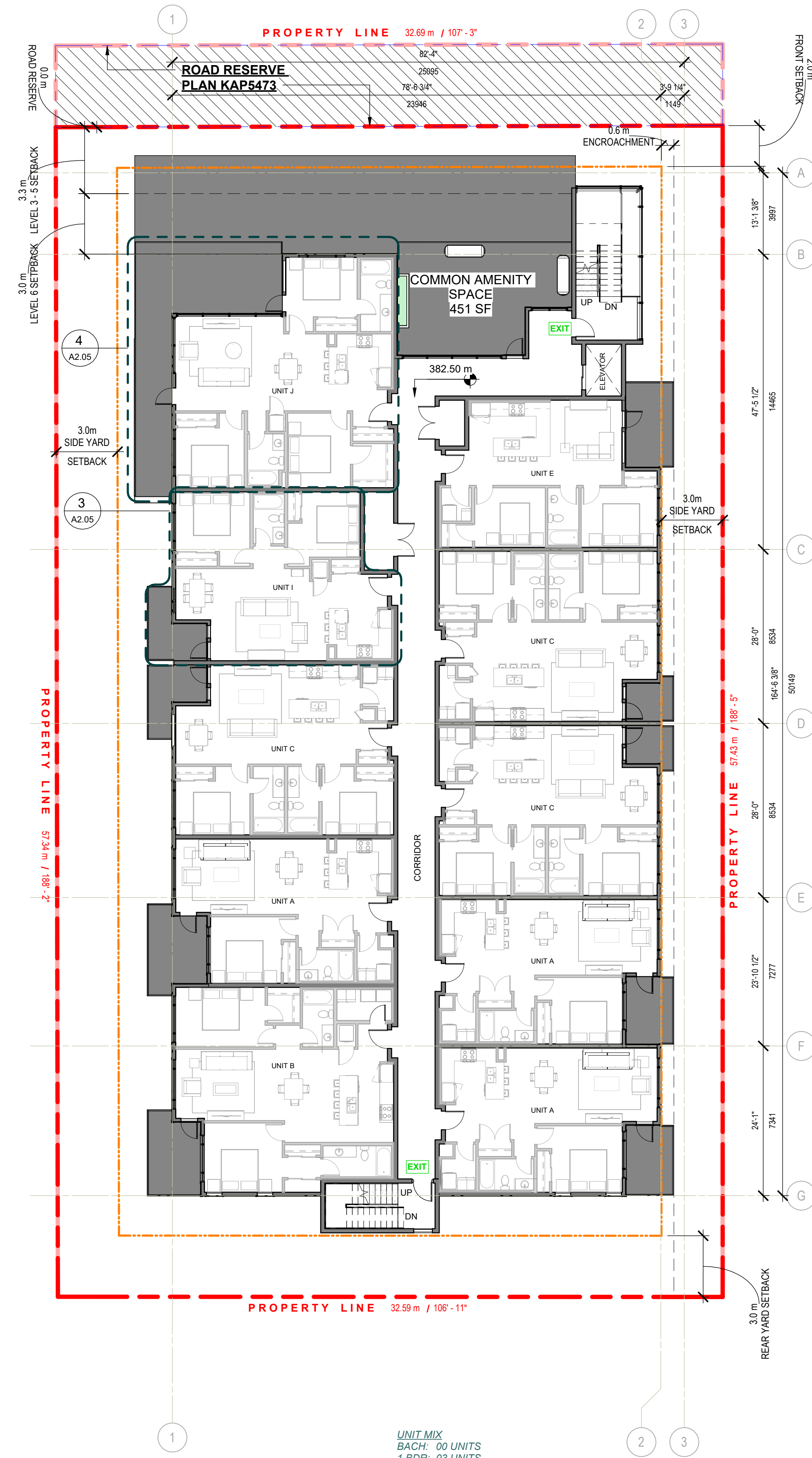
1 FLOOR PLAN - LEVEL 6 & ROOF 1 : 150 UNIT MIX: BACH: 00 UNITS 1 BDR: 03 UNITS 2+BDR: 07 UNITS TOTAL: 10 UNITS TOTAL LEVEL 6 LIVING AREA (FOR FAR CALCULATION): 9062 SF PRIVATE OPEN SPACE AT LEVEL 4 COMMON AMENITY: 451 SF
