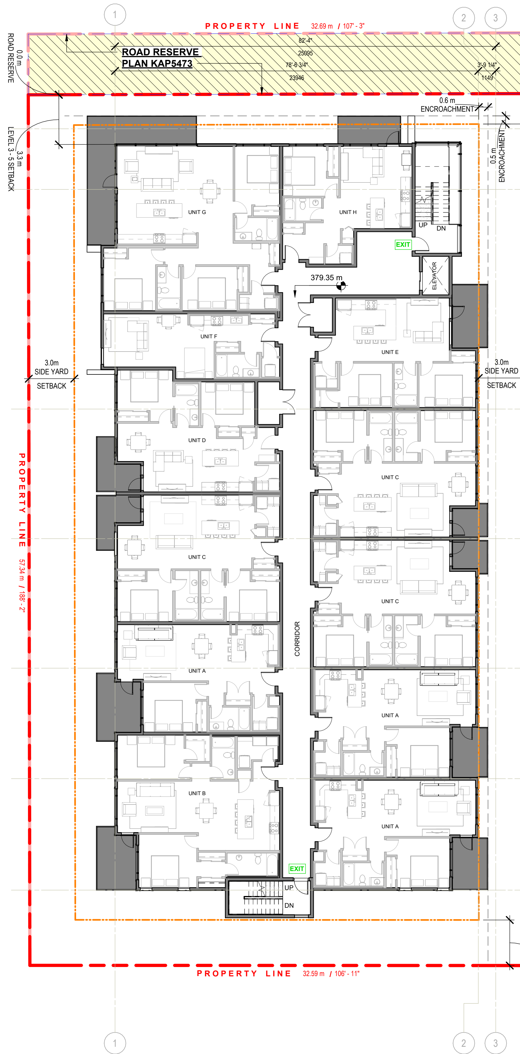
3 FLOOR PLAN - LEVEL 5 1 : 150 UNIT MIX BACH: 01 UNITS 1 BDR: 04 UNITS 2+BDR: 07 UNITS TOTAL: 12 UNITS TOTAL LEVEL 5 LIVING AREA (FOR FAR CALCULATION): 10237 SF PRIVATE OPEN SPACE AT LEVEL 4
