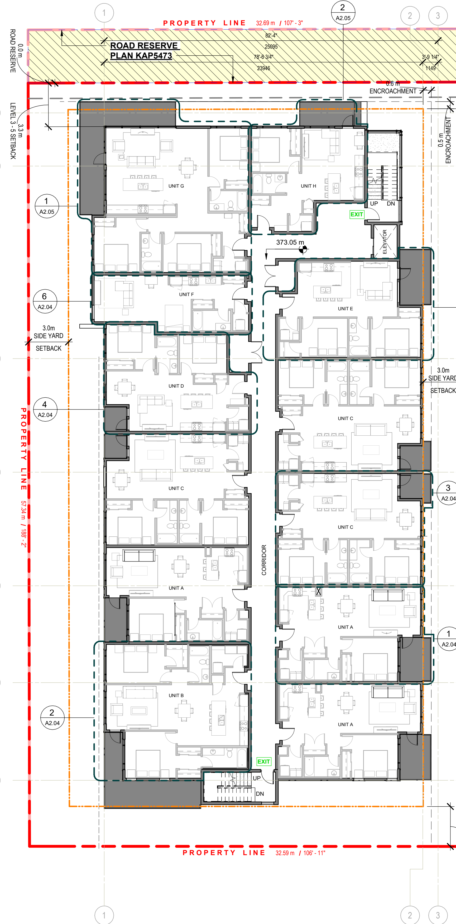
1 FLOOR PLAN - LEVEL 3 1 : 150 UNIT MIX BACH: 01 UNITS 1 BDR: 04 UNITS 2+BDR: 07 UNITS TOTAL: 12 UNITS TOTAL LEVEL 3 LIVING AREA (FOR FAR CALCULATION): 10237 SF PRIVATE OPEN SPACE AT LEVEL 3
